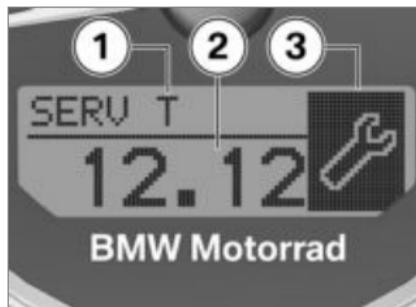
When a service is due within one month, symbol for service due **3** and service due date **2** are displayed. **SERV T 1** appears briefly on the display after the Pre-Ride-Check completes.
