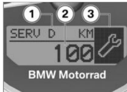
When a service is due within 1000 km, symbol for service due **3** and countdown distance **2** are displayed and the countdown proceeds in steps of 100 km. **SERV D 1** appears briefly on the display after the Pre-Ride-Check completes.
