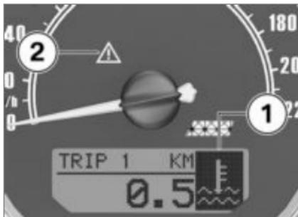
Warnings that do not have warning lights of their own are indicated by a warning symbol **1** appearing in the multifunction display in combination with 'Gen-
